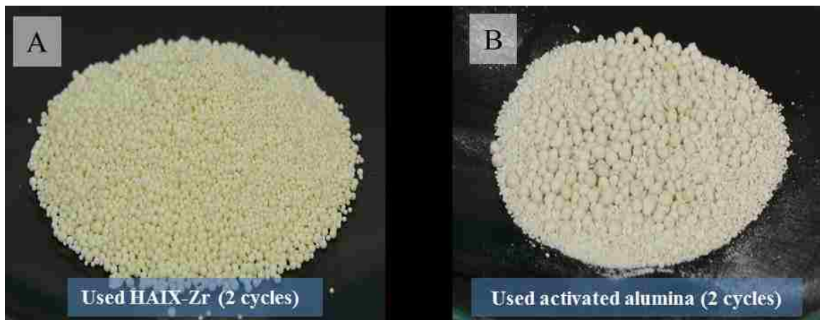
Figure 5.9 Comparison of XRD diffractograms between used HAIX-Zr and activated alumina (AA) after 3 cycles of sorption/desorption for fluoride removal column run experiment and mechanical strength of used (A) HAIX-Zr and (B) Activated Alumina
